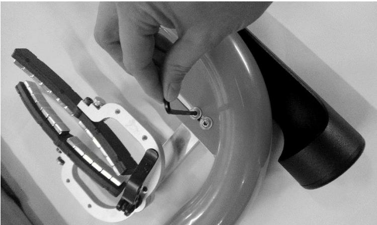
4. Use the position of your old Resistance Unit as an initial guide for mounting the new Resistance Unit. Attach your Halcyon Resistance Unit to the Frame, tightening the 2 Mounting Bolts just enough to prevent any movement of the Resistance Unit until you perform the alignment steps.
